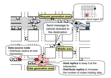
Figure 4: Deployment of fixed nodes
