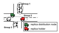
Figure 3: RD method: Grouping vehicles based on their traveling directions
