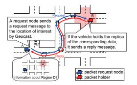
Figure 1: System configuration of Sharing Objects with Location information on Ad-hoc networks (SOLA)
