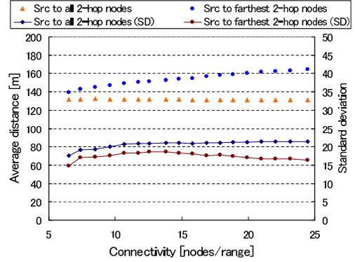
Figure 8: Average distance and standard deviation of all 2-hop nodes and the farthest 2-hop nodes
