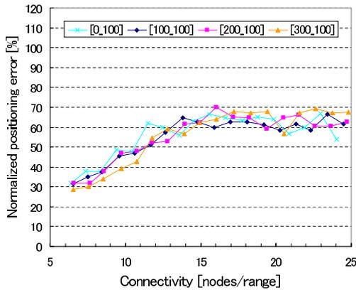
Figure 10: Normalized positioning error for the various obstruction scenarios
