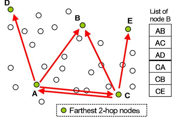
Figure 5: Illustration of matching regular triangles for node  $B$ . The list shows the received farthest 2-hop nodes list of node  $B$  after receiving  $\text{TRI\_NOTICE}$  packets from node  $A$ ,  $C$
