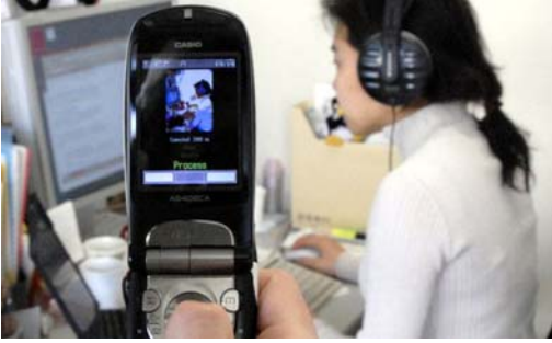
Figure 8: EZ mobile application for image retrieval. Color has been quantized and the image is to be sent to the database.
