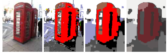
Figure 1: Segmentation example. From left to right: original image; the result of color categorization; after applying the occlusion N-sieve; and the resulting regions represented by their mean color.
